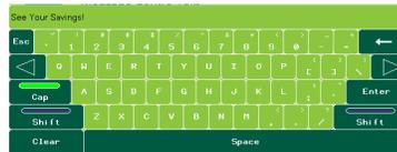
Type new text using the pop-up keyboard. Touch **Enter** to save or **ESC** to cancel and return to the **Primary Toolbox** window.
