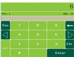
Using the pop-up keyboard, *type* the number for the time. Touch **enter** to return to the Motor Starter Schedule window.
