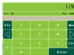
Type the new setting (in seconds) using the pop-up keyboard. Touch **enter** to return to **Primary Toolbox** window.
