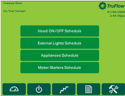
The automatic schedule is useful if you would like your exhaust system, external lights, appliances and motor starters to turn on and off at a set time each day. You can set up a different automatic start and stop time for each day of the week, and each lighting zone/appliance/motor starter. You will need to set an automatic start/stop time for every day of the week you will *not* be operating the exhaust system in manual (HAND) mode.
