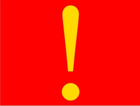
When a message that requires immediate attention or action occurs, the screen will change to red with a yellow exclamation mark. These types of alarm include certain drive errors where the VFD cannot reset automatically, and catastrophic equipment failures (exhaust fan or makeup air unit not running).
