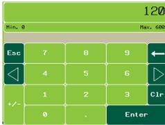
Using the pop-up keyboard, *type* the length of time (in seconds) after the exhaust system has been turned off before the wash sequence will run.
