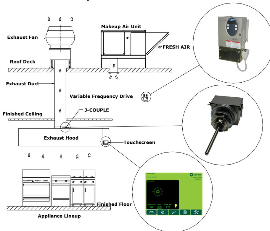
TruFlow measures heat from the appliances and automatically adjusts fan speeds throughout the day, giving you the precise amount of exhaust at all times. As more cooking appliances are used the exhaust and supply volume increase; as fewer appliances are used, the exhaust and supply volume decrease.
