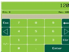
Using the pop-up keyboard, *type* the length of time (in seconds) after the wash sequence should run for.
