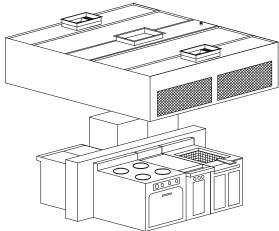
VARIFLOW BAFFLE for adjustable exhaust air flow. The VORTEX BAFFLE is removable for periodic cleaning.
