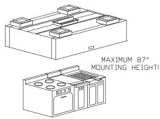
The *Dynaflow* design provides the complete commercial kitchen ventilation package. The *Dynaflow hood* exhaust calculations are based on the appliance below the hood. Heated and/or cooled fresh air ducting is connected to the two supply duct collars on the top, front of the hood. The fresh air flows into these connections through the supply fire damper and to the *Dynaflow* chamber. Fresh is directed to two locations within the perimeter of the cooking appliances.
