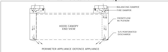
The fresh air discharges through a fusible link fire damper into the MJ Plenum. The air is then discharged from the bottom through the MJ-Grill. The air can be proportioned between the appliances and the chef area by adjusting the comfort tuning dial. In the middle of the Chef Region is an adjustable Comfort Tuning Dial. The Comfort Tuning Dial proportions the amount of air to the Chef Region.
