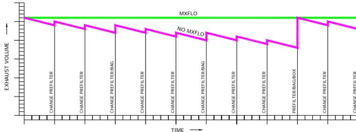
**Maxflow:** The RPD-KD11-TS provide Maxflow for the KES filters. Maxflow extends the life of each filter by monitoring the inlet pressure. When the filters collect grease the pressure drop increases, the exhaust volume decreases and the inlet static decreases. Maxflow increases the drive speed to hold the inlet static pressure and the exhaust volume constant
