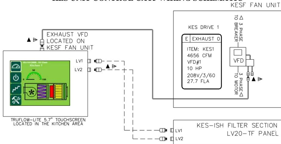
**Control wiring:** RPD-KD11-TS control wiring is 3 CAT5 cables to the KES filter LV20-TS and 1 CAT5 cable to the KESF fan section drive. The LV20-TS panel contains the 4 transducer to monitor static pressure across each filter and the KES inlet.
