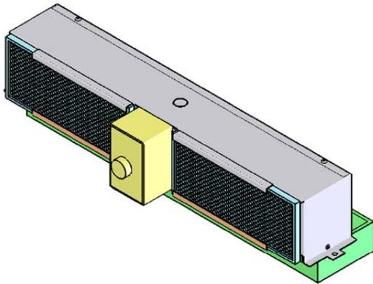
The MJ blower assembly is located on top of the MJ plenum. Each hood has one or more MJ Blower assemblies. To adjust the air flow of the MJ blower rotate the rheostat in the middle of the MJ blower assembly. Rotating the knob clockwise increases the air flow and rotating the knob counter clockwise decreases the amount of air into the plenum. Adjust the knob until the correct velocity is measured one the MJ Grill appliance discharge.
