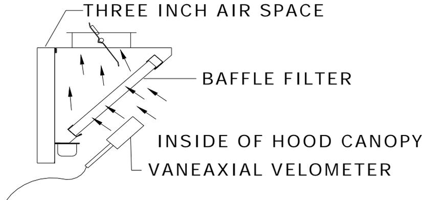
*Measuring baffle filter exhaust Air with Vanaxial velometer
