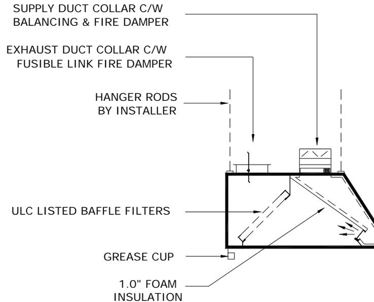
*Cross Section of Filter Hood Model FD-B-MI
