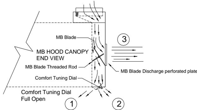
Each of the three regions must be measured to ensure proper hood operation. The Appliance Region, the Chef Region and the Kitchen Ambient Region as shown in the schematic Figure 28
