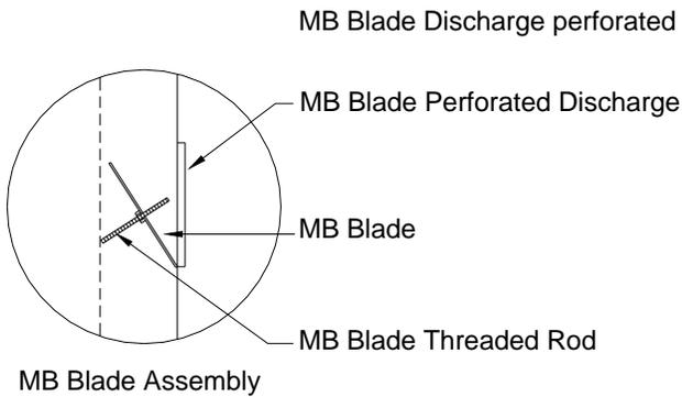
Measuring MB Blade Perforated Discharge
