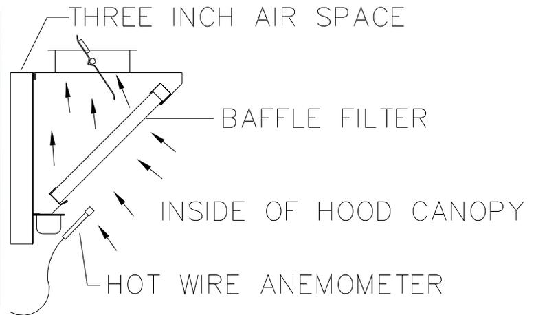
Measure velocity here at the bottom of each slot. Average the velocities across the filter and determine the CFM using Chart No. 2. See figure 25 for location of the Pitot tube or hot water anemometer when measuring the velocity
