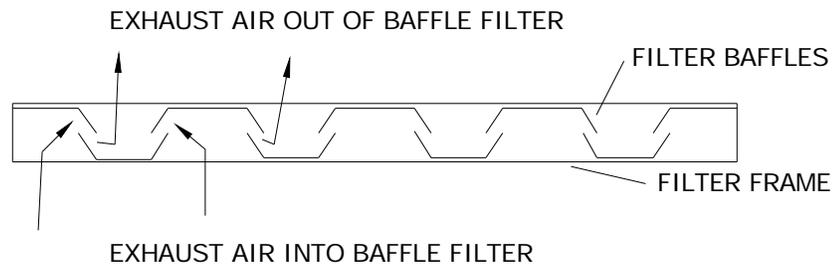
*Cross Section of Baffle Filter
