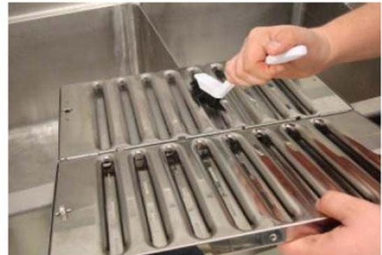
Cascade's locking handles open up the hinged design, allowing a wide-open cleaning access.
