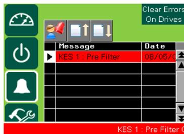
The window displays the latest alarm message including the date, time, state and whether the alarm has been acknowledged.
