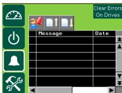
The **Alarm Status** window provides a list of current and previous alarms that have been recorded by the touchscreen. A few of the recorded alarms are filters requiring changing, power outages, and high temperature. You will need to go to this screen to clear an alarm. The red alarm message indicates an active alarm, a green alarm message indicates a cleared alarm, and a yellow alarm message indicates the alarm is still active, but has been acknowledged.
