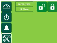
The **Primary Toolbox** window allows you to make changes to the date, time, automatic opening and closing times, along with the time to dashboard, odour spray timer and waterwash timer. The window shown left is the Primary Toolbox before you log in. After you are logged in, you will have the options shown on the right screen.
