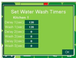
Press the dark green field next to **Delay 1**. Type the new length of time (in seconds) the exhaust system will be off before the first wash system's cycle begins. Press **enter**.
