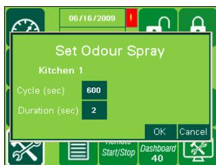
Press the dark green field next to **Cycle**. Type the new length of time (in seconds) between sprays using the pop-up keyboard.
