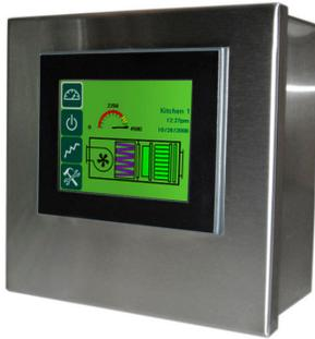
Your exhaust system is operated through a touchscreen control panel. You can turn the system on, off, set up an automatic start/stop schedule, and monitor the status of the KES filters all through the touchscreen. The touchscreen also keeps a record of system alarms that are useful for service technicians to diagnose and correct problems.
