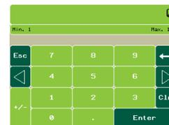
Press the dark green field next to **Duration**. Type the new length of time (in seconds) the spray discharges. The higher this number, the longer the spray.
