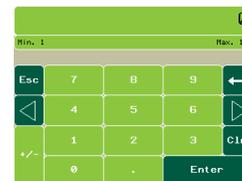
Press the dark green field next to **Wash 1**. Type the new length of time (in seconds) the first wash system's cycle will run.
