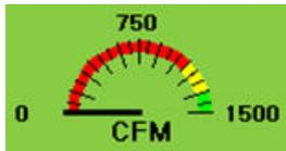
**Operating CFM Dial** indicates the current operating CFM. When the filters become so clogged that the motor can no longer compensate, this dial will drop down into the red section. Be sure to change filters *before* the system shuts down.
