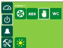
The **Power** window provides access to the exhaust components controlled by the touchscreen panel. You can turn on and off the KES, change the makeup air between summer and winter mode, and access the filter use graph.
