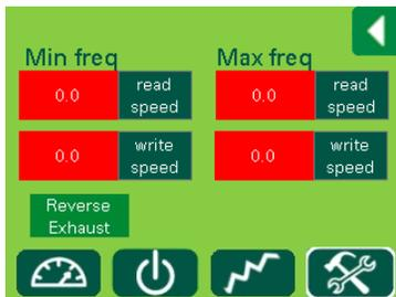
Touch **read speed** for Min freq. The field will turn pink for several seconds and then display the current minimum operating frequency on the drive.
