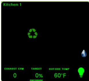
The wash cycle will run when the exhaust fan is turned OFF.
