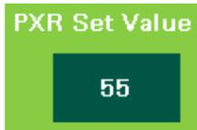
*Touch the dark green field with the PXR set value. Using the pop-up keyboard, change the PXR set value. Touch **Enter** on the pop-up keyboard, then **OK** to exit.*
