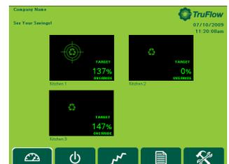
The **Power Window** provides access to all of the exhaust components controlled by the TruFlow. These include canopy lights, fan on/off, summer/winter and override settings.
