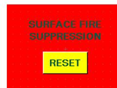
Typical fault displayed on Dashboard window after surface fire suppression activates.
