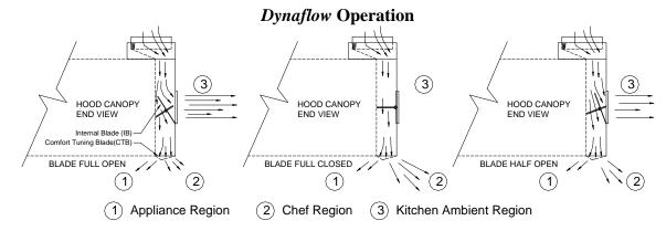
The internal blade (IB) is adjusted to direct fresh air between the Kitchen Ambient (3) Region, the Appliance (1) Region, and Chef(2) Region. The Comfort Tuning Blade (CTB) is adjusted to direct fresh air between the Appliance (1) Region and the Chef(2) Region. The complete kitchen ventilation system is always balanced. The IB and CTB are adjustable
