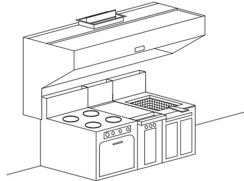
Introducing supply air back into the kitchen is good engineering practice. An adequate supply of fresh air eliminates cold drafts, and hot spots, enhances the capture capability of the filter hood and results in a more comfortable kitchen environment. A heated supply air volume up to 80% of the total exhaust is recommended
