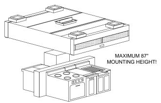
duct collars on the top, front of the hood. The fresh air enters the fire damper in each supply duct connection and then discharges into the *Dynaflow* plenum. Within the plenum the fresh air is routed to three (3) regions within the boundaries of the appliances.
