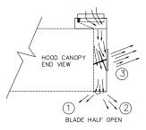
The internal blade (IB) is adjusted to direct fresh air between the Kitchen Ambient (3) Region, the Appliance (1) Region, and Chef(2) Region. The Comfort Tuning Blade (CTB) is adjusted to direct fresh air between the Appliance (1) Region and the Chef(2) Region. The complete kitchen ventilation system is always balanced. The IB and CTB are adjustable every 24" (610mm) along the length of the Dynaflow hood to
