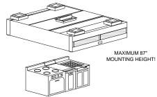
and/or cooled fresh air ducting is connected to the two supply duct collars on the top, front of the hood. The fresh air enters the fire damper in each supply duct connection and then discharges into the *Dynaflow* plenum. Within the plenum the fresh air is routed to three (3) regions within the boundaries of the appliances.
