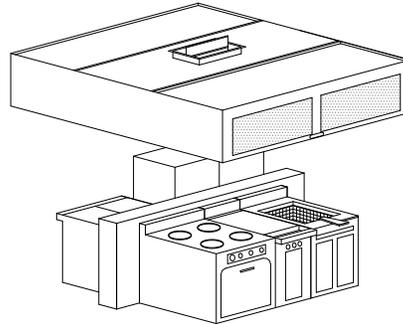
cooking equipment under the ventilator. An exhaust flow rate between 300 and 700 CFM/ft (465 and 1085 l/s/m) is required for most hoods. Heated fresh air is discharged out the front of the hood canopy for MP and MG types. Fresh air volume of 80% of the total exhaust is recommended for heated makeup air systems. Refer to the *Ventilator Engineering Manual* for supply air volume calculations.
