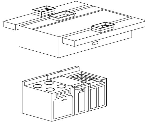
equipment under the filter hood. An exhaust flow rate of between 150 to 400 CFM/ft (233 to 620 l/s/m) is satisfactory for most installations. Directing the make up air down, from the front of the hood provides continuous air movement, directed towards the cook.
