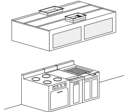
equipment under the filter hood. An exhaust flow rate of between 150 to 400 CFM/ft. (233 to 620 l/s/m) is satisfactory for most installations. Directing the make-up air through the front of the hood provides the correct air quantity and excellent distribution within the kitchen.
